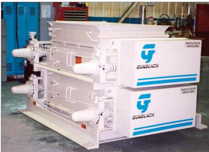
Figure 2. A Gundlach four roll crusher used for sizing coal and coke for fuel in
